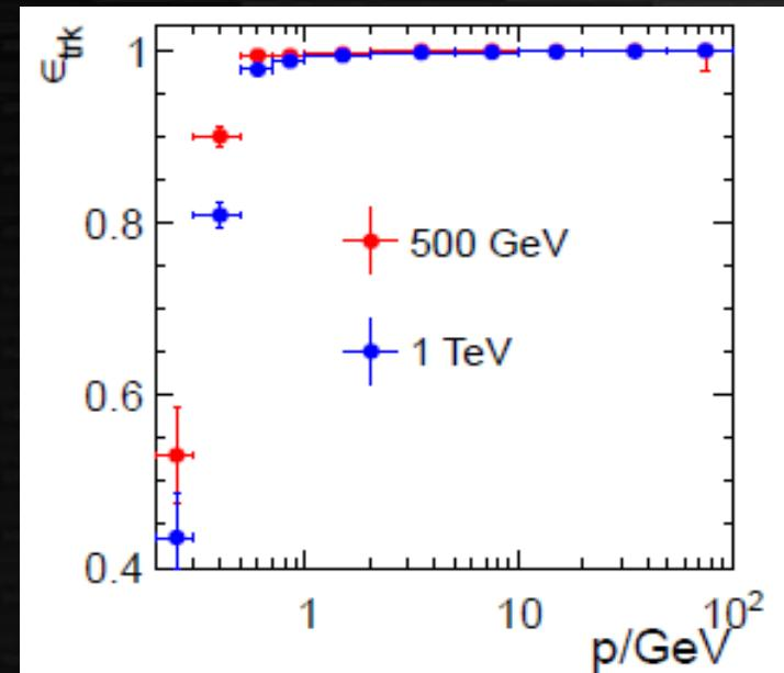
Taikan: tracking efficiency of  $t\bar{t} \rightarrow 6$  jet events
