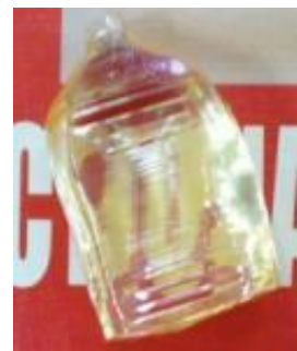
Ø25×60 mm 2010 Low-thermal-gradient Czochralski technique
