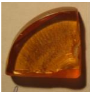
Ø15×40 mm Ø30×15 mm 2008 Czochralski and Kyropoulos methods
