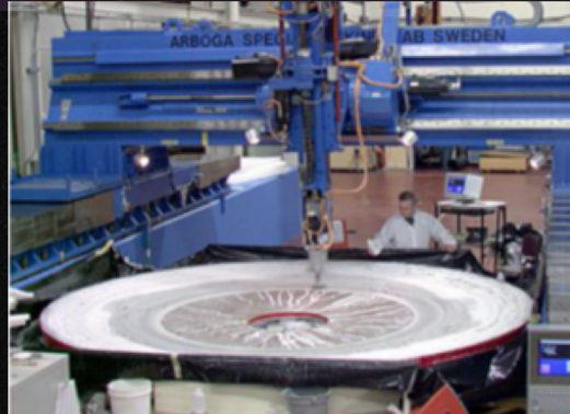
4.2m mirror for the Southern Astrophysical Research Telescope
