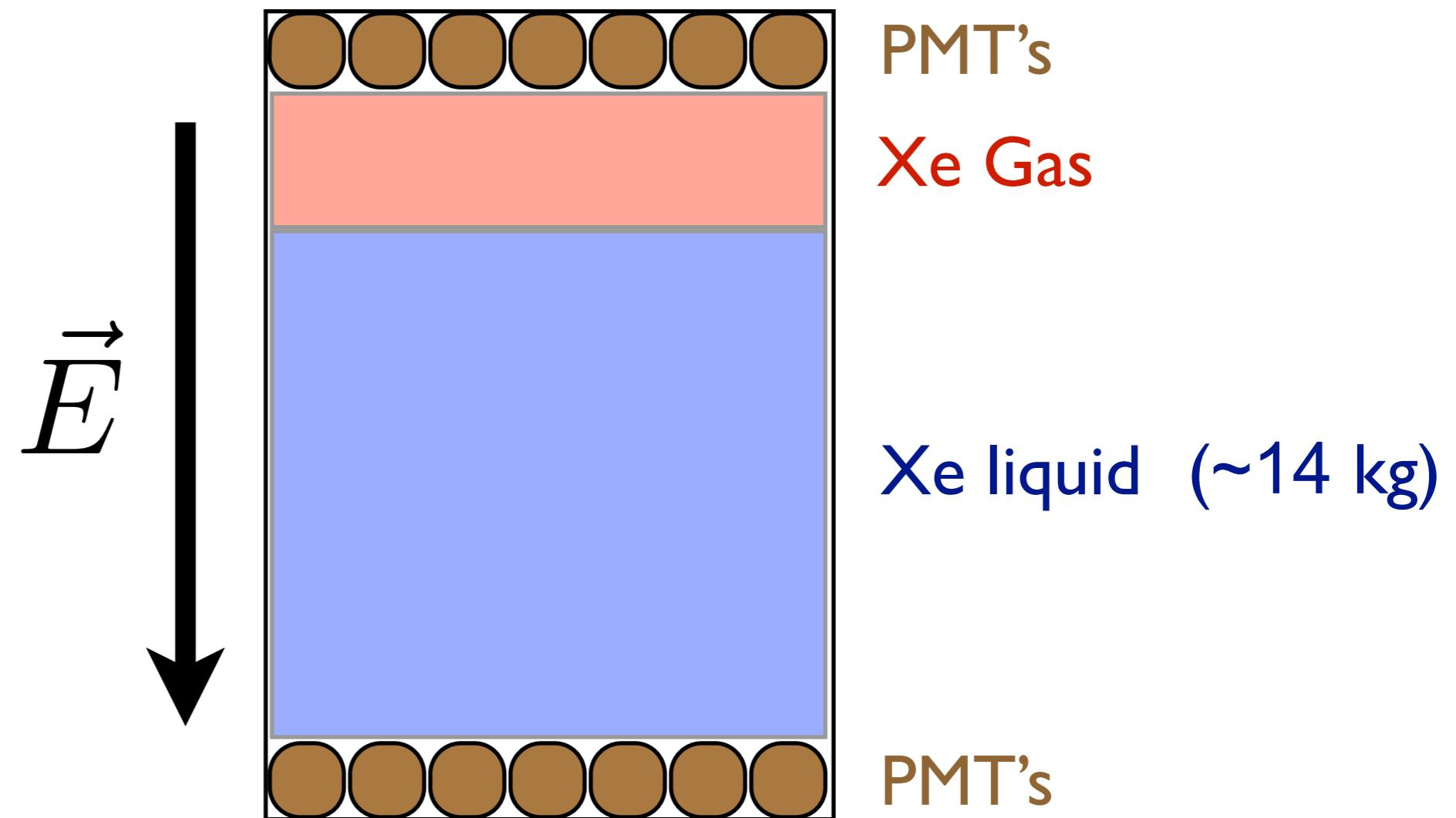
two-phase xenon time projection chamber
