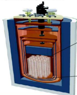
Single dilution refrigerator -10 mk
