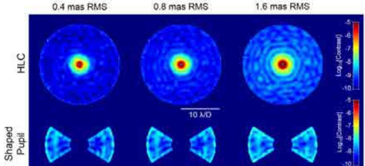
Figure 3-26: Log scale contrast maps for the HLC and SPC, in the presence of different levels of post-LOWFS jitter. Both designs show good tolerance to jitter.
