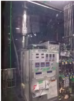
Xe distillation + filtration (charcoal, sintered metal, 3nm PTFE)+ getter
