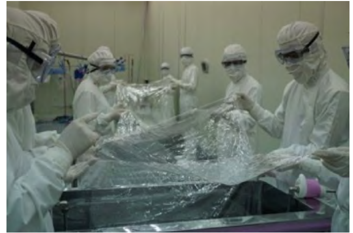
Washing nylon films (Ultra-pure water + ultrasonic machine)
