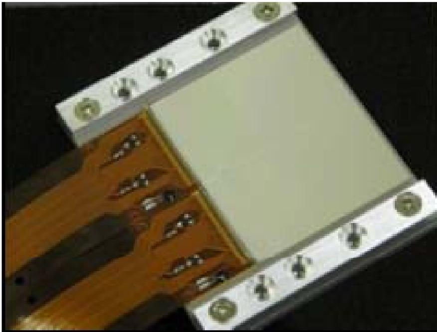
X-ray CCD chip by Hamamatsu Photonics
