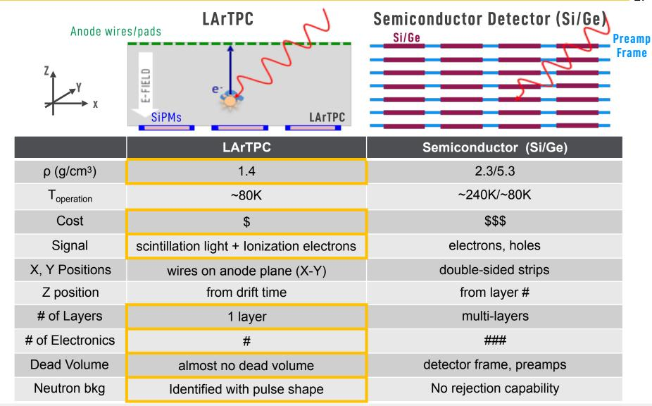
LARTPC IS COST-EFFECTIVE AND EASILY EXPANDABLE TO A LARGER-SCALE, MUCH LESS CHANNELS/ELECTRONICS REQUIRED, ALMOST NO DEAD VOLUME
