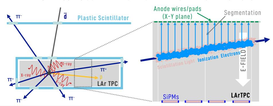
Plastic Scintillators: TOF - measure velocity and incoming angle
