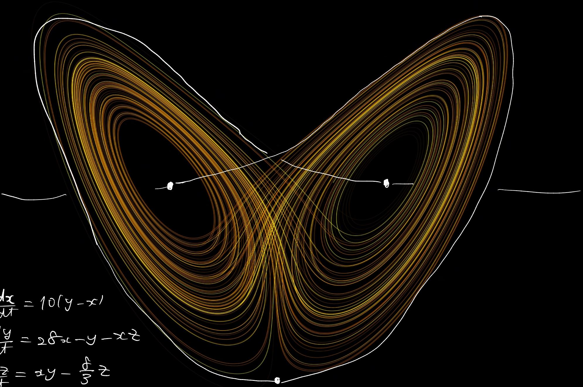
$$\left\{ \begin{array}{l} \frac{dx}{dt} = 10(y - x) \\ \frac{dy}{dt} = 28x - y - xz \\ \frac{dz}{dt} = xy - \frac{8}{3}z \end{array} \right.$$
