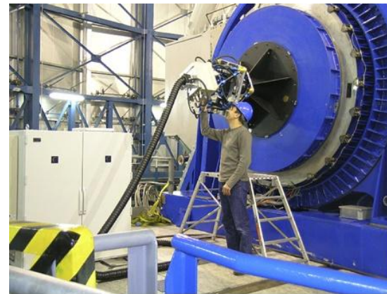
ULTRACAM Mounted on Visitor Focus of MELIPAL
