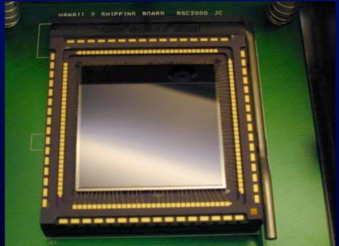
**WFCAM detector, UK Infrared Telescope**
